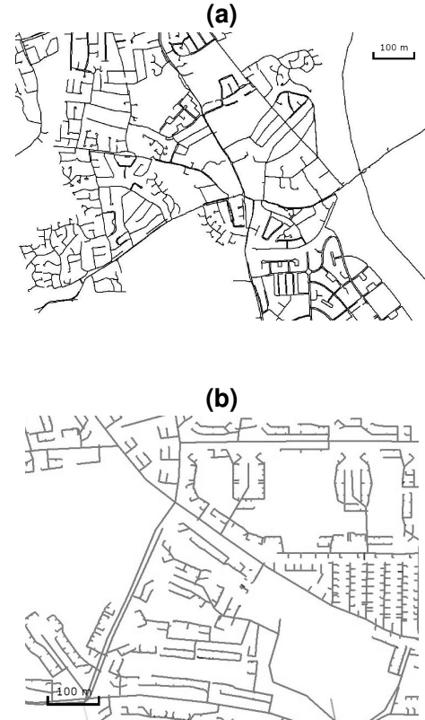
Fig. 1. Examples of (a) water distribution, and (b) wastewater pipe networks in towns in the UK.
